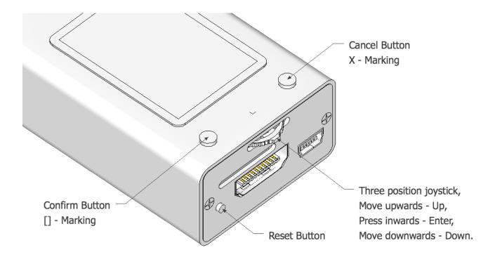
Two buttons are located on topside panel: Cancel(X) and Confirm([]) and on the right side panel the reset button and our three position joystick are located. The joystick provide functionality for up / down / select. Complete use of this buttons will be detailed for each applications, but the standard use is:
